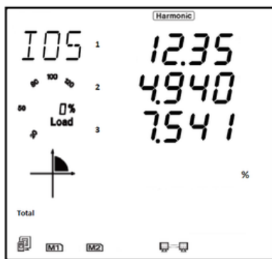
Figure 3-23 - Individual Harmonic Reading
