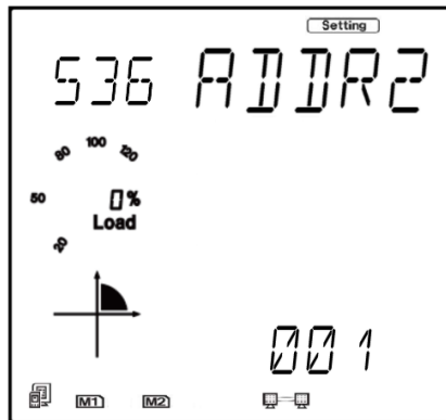
Figure 5-55 Address setting for AXM-RS485
