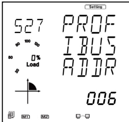
Figure 5-50 AXM-PROFI address setting on meter display
