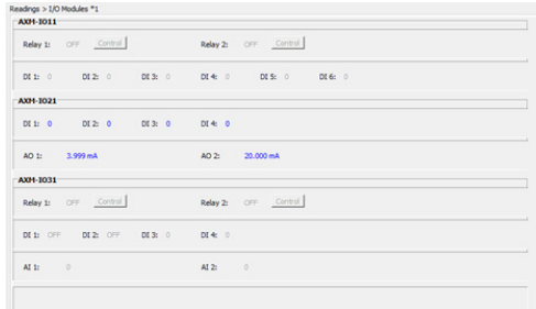
Figure 5-41 Analog Output readings on the Acuvim software
